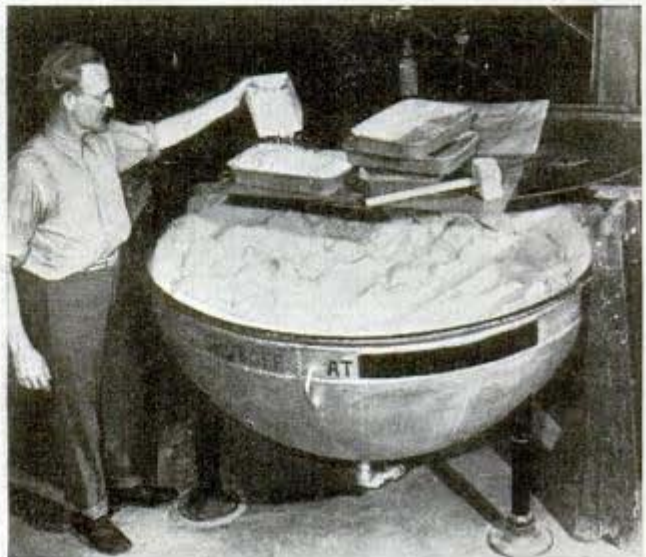
After ores have been purified to form pure tungstic oxide, the oxide powder is put into pans for drying in ovens
